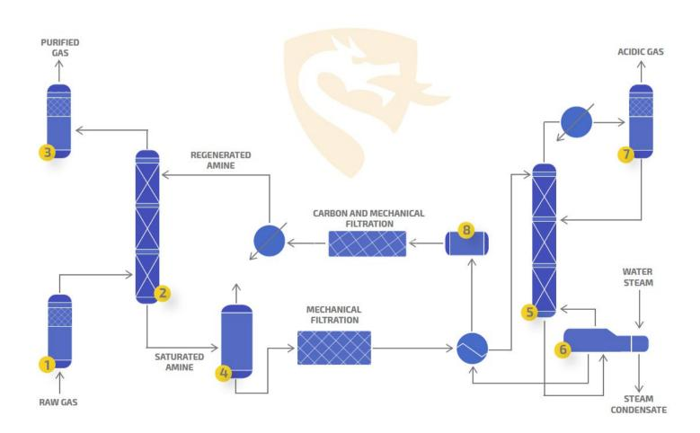
Then the vapor-gas stream enriched with H2S and CO2 exits the column and enters the air cooler, after which the gas-liquid mixture enters the reflux tank:
